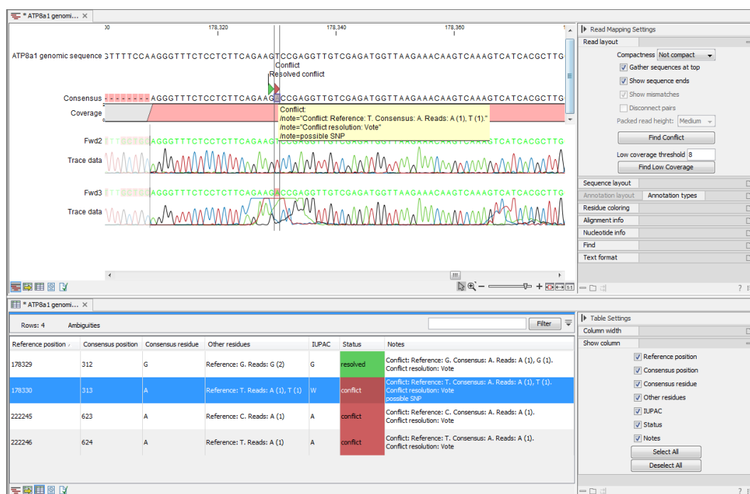
Figure 18.18: The graphical view is displayed at the top, and underneath the conflicts are shown in a table. At the conflict at position 313, the user has entered a comment in the table (to see it, make sure the Notes column is wide enough to display all text lines). This comment is now also added to the tooltip of the conflict annotation in the graphical view above.
