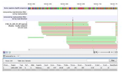
Figure 27.23: A variant that is filtered out by the Read position filter but not by the Read direction filter.
