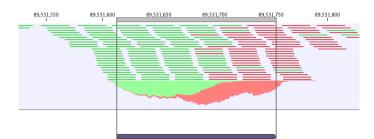
Figure 30.1: Distribution of forward (green) and reverse (red) reads around a binding site of the transcription factor NRSF.
