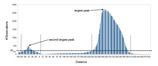
Figure 29.11: Histogram of paired distances where  $H_{avg}$  is indicated by the horizontal dashed line. There is two peaks, one is at a negative distance while the other larger peak is at a positive distance. The extended interval [k, l] for each peak is indicated by the vertical dotted lines.
