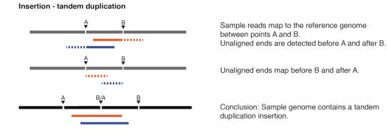
Figure 27.39: An insertion with breakpoint mapping evidence corresponding to a 'Tandem duplication'.
