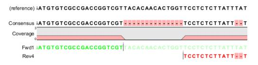
Figure 25.12: A region of zero coverage in the middle and one time coverage on each side. Note that the gaps to the very right are within the same read which means that these two positions on the reference sequence are still counted as "covered".
