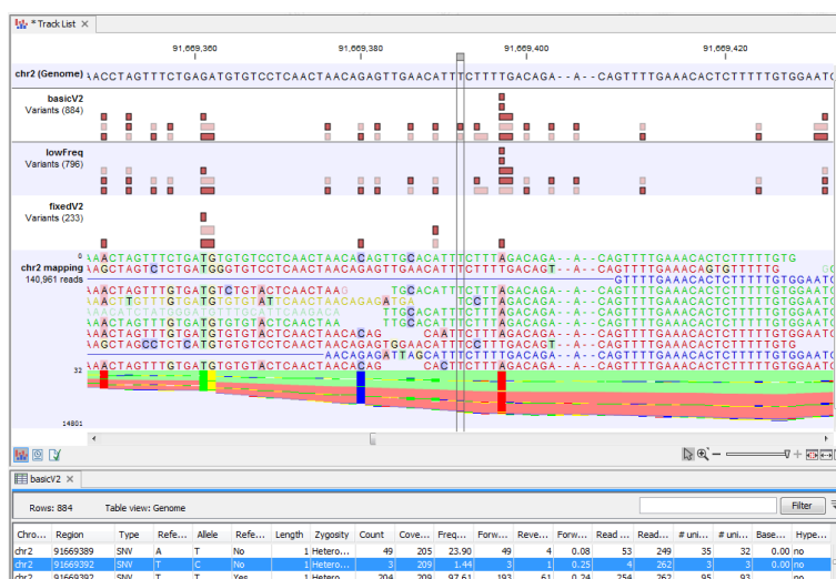
Figure 27.13: A variant is highlighted that is detected by the Basic Variant Caller but not by the Low Frequency or the Fixed Ploidy Variant Caller. The variant track for the Basic variant Caller variants is opened in the table-view at the bottom of the figure. The variant is present at a low frequency in a high coverage position, and is likely to have been caused by sequencing error.
