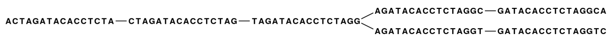
Figure 29.2: Three nodes connected, each sharing 15 bases with its neighboring node and ending with two forward neighbors.
