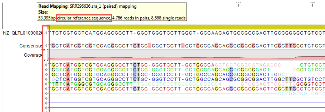
Figure 27.24: Mapping reads to a circular chromosome. Reads that are marked with double arrows at the ends are reads that map across the starting point of the sequence. The arrows indicate that the alignment continues at the other end of the reference sequence.
