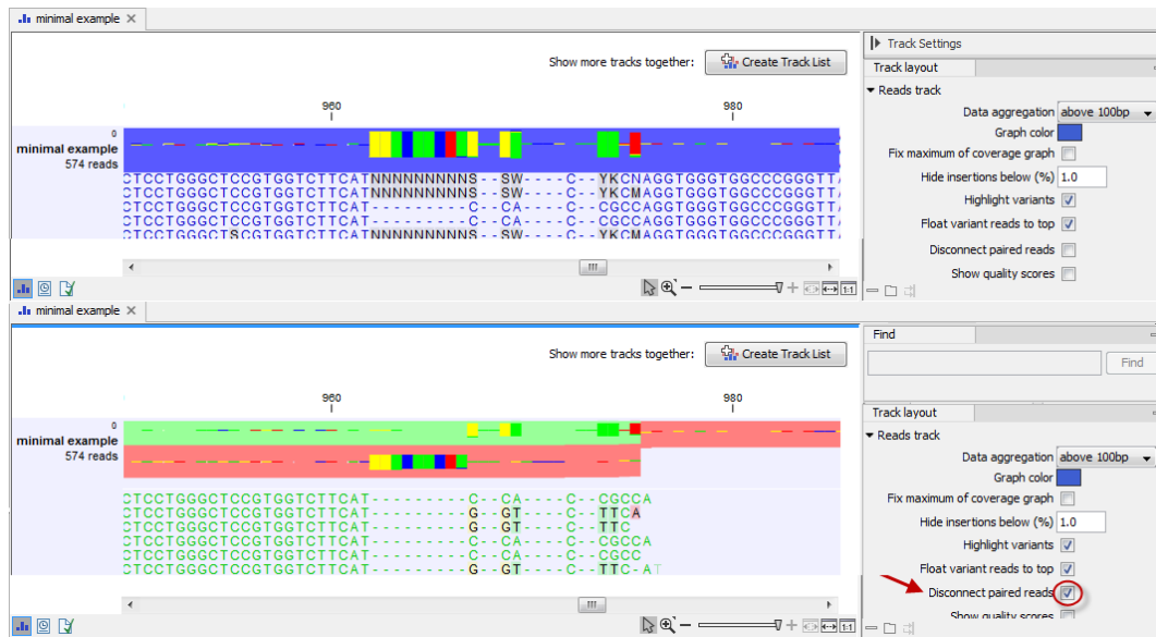
Figure 27.23: Overlapping paired reads containing discrepancies in the overlapping region. The divergent area in the overlapping read pair is marked with N's and IUPAC codes in the top part of the figure. Disconnecting the paired reads by ticking the box "Disconnect Paired Reads" in the Side Panel allows you to see the individual reads.
