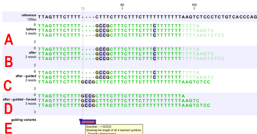
Figure 27.35: [A] Three reads are misaligned in the presence of a four nucleotide insertion relative to the reference. [B] When applying local realignment without guidance the alignment is not improved. [C] Here local realignment is performed in the presence of the guiding variant track seen in (E). This enables the algorithm to consider alternative alignments, which are accepted whenever they have significant improvements over the original (as in read three that has a comparatively long unaligned-end). [D] If the alignment is performed with the option "Force realignment to guidance-variants" enabled, the realignment will be forced to realign according to the guiding variant track shown in (E), and this will result in realignment of all three reads. [E] The guiding variant track contains, amongst others, the four nucleotide insertion.
