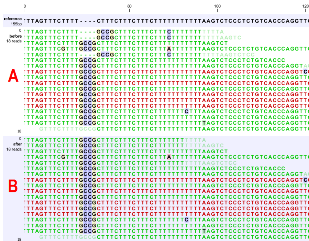
Figure 25.30: Local realignment of a read mapping produced with the 'local' option. [A] The alignments of the first, second, and fifth read in this read mapping do not support the four-nucleotide insertion supported by the remaining reads. A variant detection tool might be tempted to call a heterozygous insertion of four nucleotides in one allele and heterozygous replacement of four nucleotides in a second allele. [B] After applying local realignment, the first, second, and fifth read consistently support the four-nucleotide insertion.
