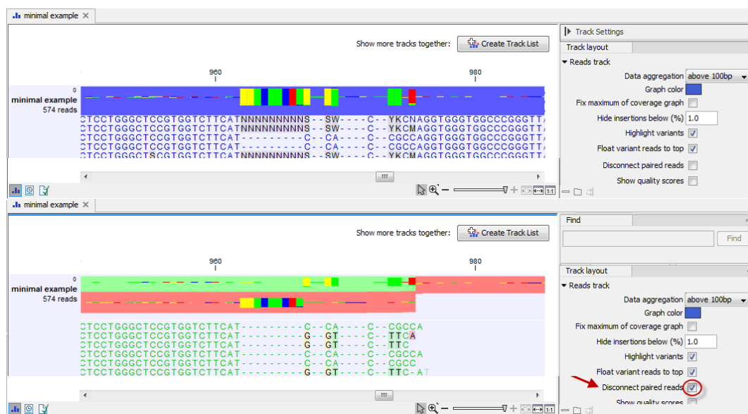
Figure 25.22: Overlapping paired reads containing discrepancies in the overlapping region. The divergent area in the overlapping read pair is marked with N's and IUPAC codes in the top part of the figure. Disconnecting the paired reads by ticking the box "Disconnect Paired Reads" in the Side Panel allows you to see the individual reads.
