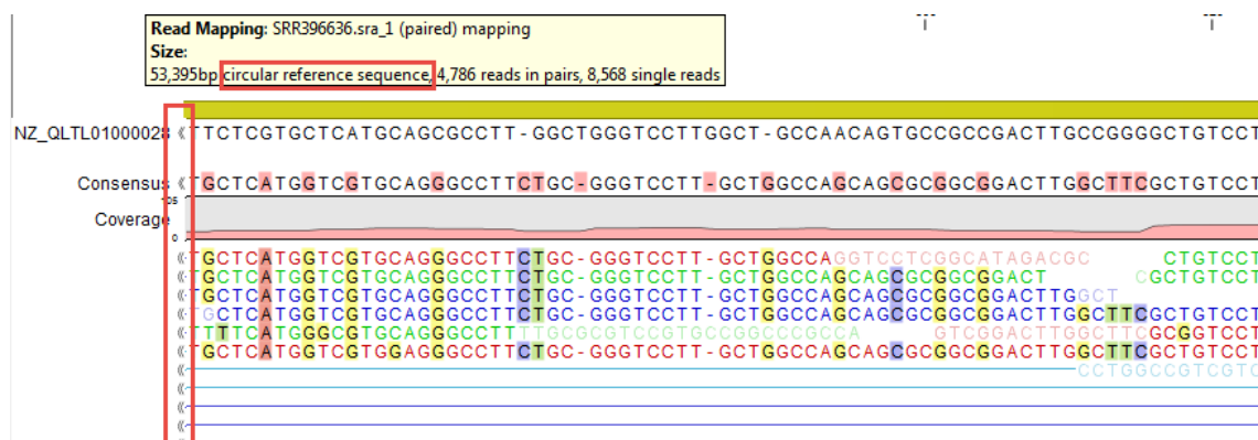
Figure 25.23: Mapping reads to a circular chromosome. Reads that are marked with double arrows at the ends are reads that map across the starting point of the sequence. The arrows indicate that the alignment continues at the other end of the reference sequence.
