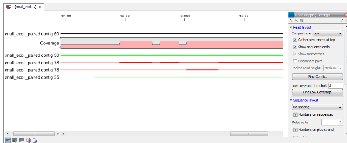
Figure 2.6: The contigs aligned to themselves. In this example, the top match is the contig itself with a perfect alignment. There is a big overlap with contig 78, which seems to share a region with contig 50. The bottom match from contig 35 is faded which mean that contig 35 does not match contig 50 in the region shown but there is a match somewhere else.
