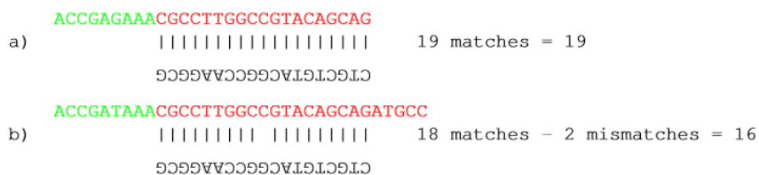
Figure 19.10: An adapter defined as CTGCTGTACGGCCAAGGCG searching on the minus strand. Red is the part that is removed and green is the retained part. The retained part is 3' of the match on the minus strand, just like matches on the plus strand.
