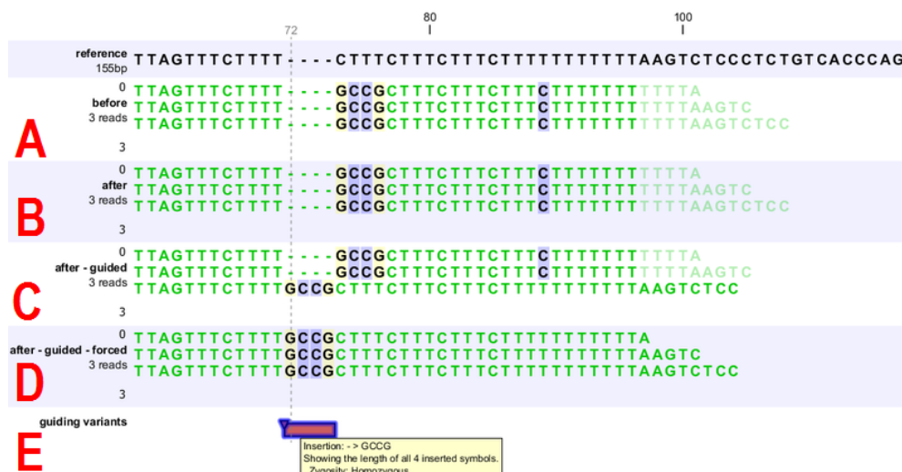
Figure 21.26: [A] Three reads are misaligned in the presence of a four nucleotide insertion relative to the reference. [B] When applying local realignment without guidance the alignment is not improved. [C] Here local realignment is performed in the presence of the guiding variant track seen in (E). This enables the algorithm to consider alternative alignments, which are accepted whenever they have significant improvements over the original (as in read three that has a comparatively long unaligned-end). [D] If the alignment is performed with the option "Force realignment to guidance-variants" enabled, the realignment will be forced to realign according to the guiding variants track shown in (E), and this will result in realignment of all three reads. [E] The guiding variants track contains, amongst others, the four nucleotide insertion.
