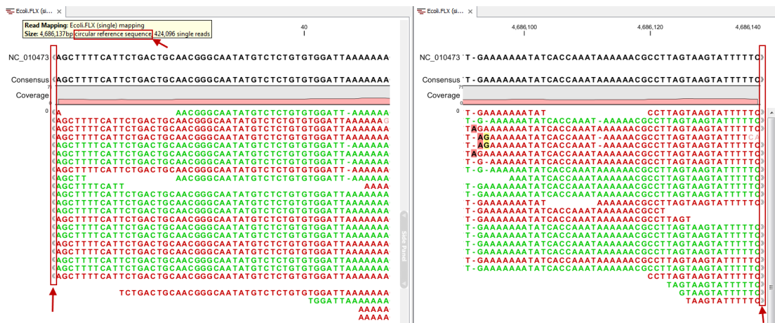
Figure 21.22: Mapping reads to a circular chromosome. Reads that are marked with double arrows at the ends are reads that map across the starting point of the sequence. The arrows indicate that the alignment continues at the other end of the reference sequence.
