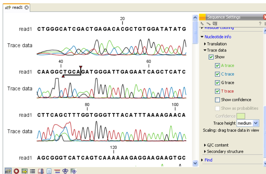
Figure 31.3: A sequence with trace data. The preferences for viewing the trace are shown in the Side Panel.
