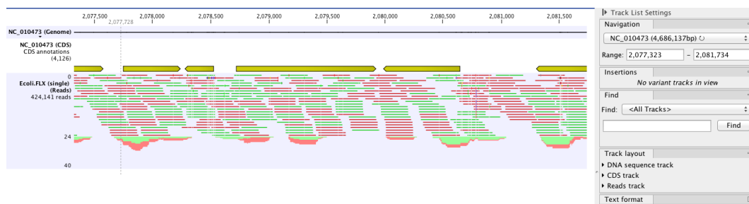
Figure 9: Track list including reference, CDS annotation track and mapped reads. The read colors are green (forward) and red (reverse) by default.
