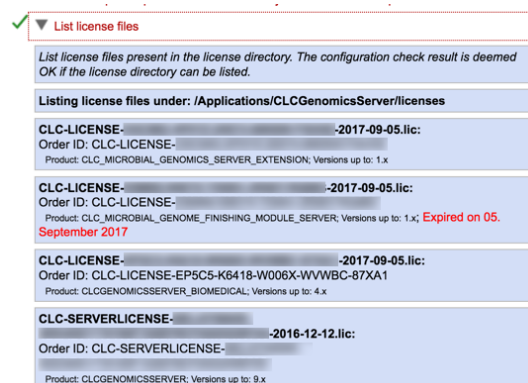
Figure 15.2: Click on the List license files item in the report to see the list of the license files found in the licenses subfolder of the installation area. Products and versions supported are reported, and any expired license is noted with red text.
