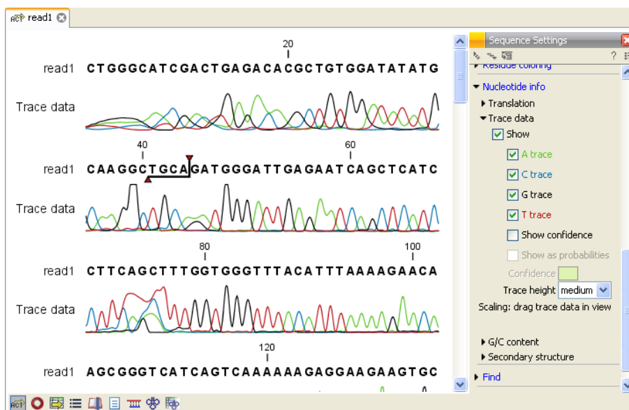
Figure 21.3: A sequence with trace data. The preferences for viewing the trace are shown in the Side Panel.
