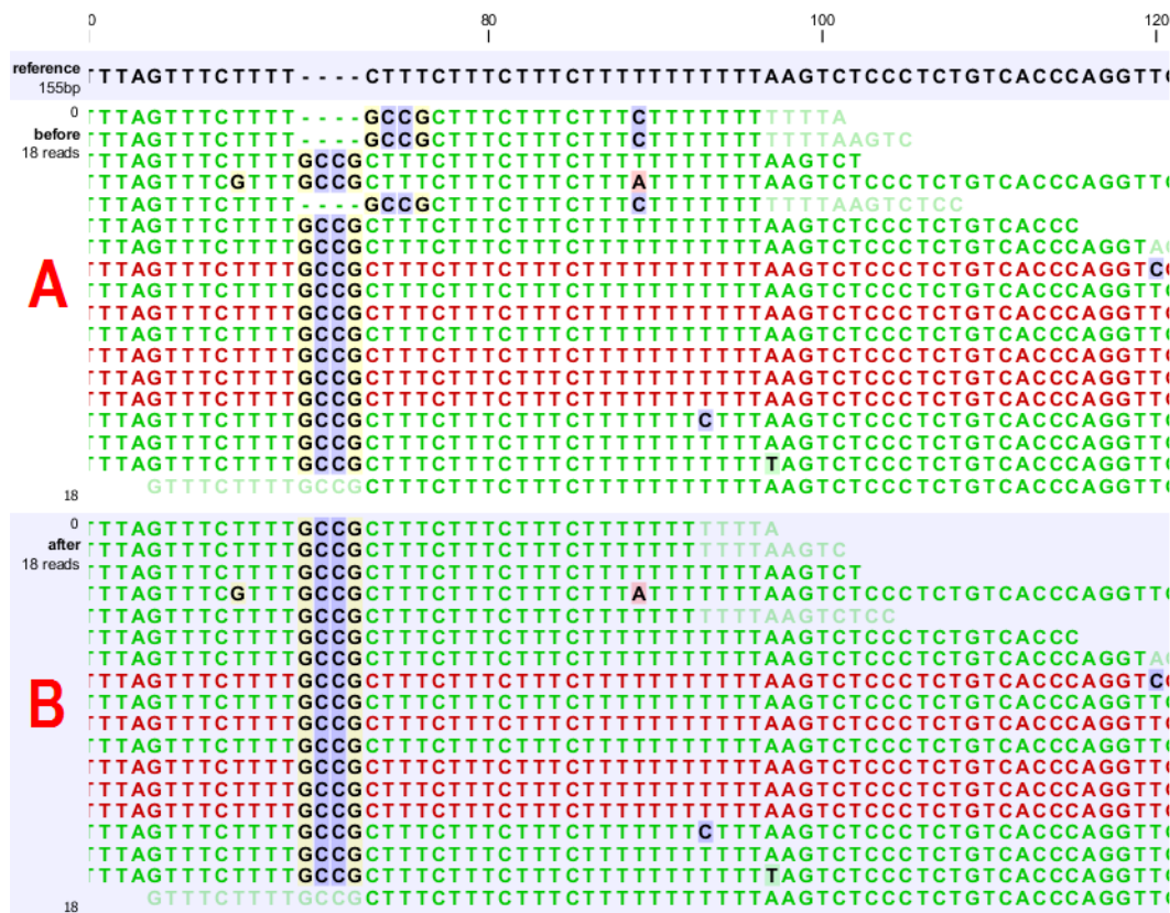
Figure 24.40: Local realignment of a read mapping produced with the 'local' option. [A] The alignments of the first, second, and fifth read in this read mapping do not support the four-nucleotide insertion supported by the remaining reads. A variant caller might be tempted to call a heterozygous insertion of four nucleotides in one allele and heterozygous replacement of four nucleotides in a second allele. [B] After applying local realignment, the first, second, and fifth read consistently support the four-nucleotide insertion.
