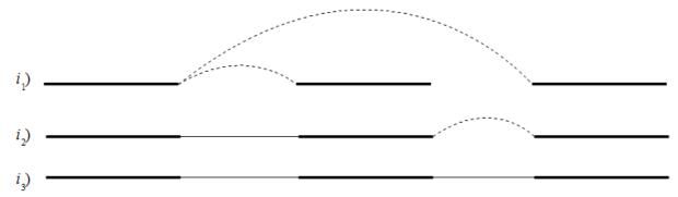
Figure 29.12: Performing iterative scaffolding of the shortest gaps allows long pairs to be optimally used.  $i_1$  shows three contigs with dashed arches indicating potential scaffolding.  $i_2$  is after first iteration when the shortest gap has been closed and long potential scaffolding has been updated.  $i_3$  is the final results with three contigs in one scaffold.
