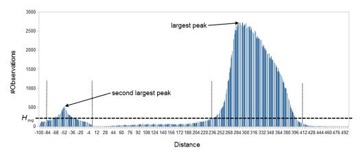
Figure 29.11: Histogram of paired distances where  $H_{avg}$  is indicated by the horizontal dashed line. There is two peaks, one is at a negative distance while the other larger peak is at a positive distance. The extended interval [k, l] for each peak is indicated by the vertical dotted lines.
