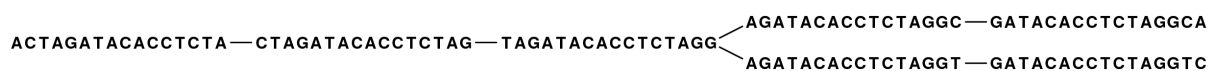
Figure 28.2: Three nodes connected, each sharing 15 bases with its neighboring node and ending with two forward neighbors.
