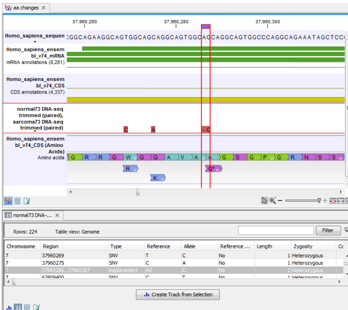
Figure 27.42: The resulting amino acid changes in track and table views. When the variant table has been opened by double-clicking on the text found in the left side of the View Area, the variant table and the variant track are linked. When clicking on an entry in the table, this position will be brought into focus in the variant track.
