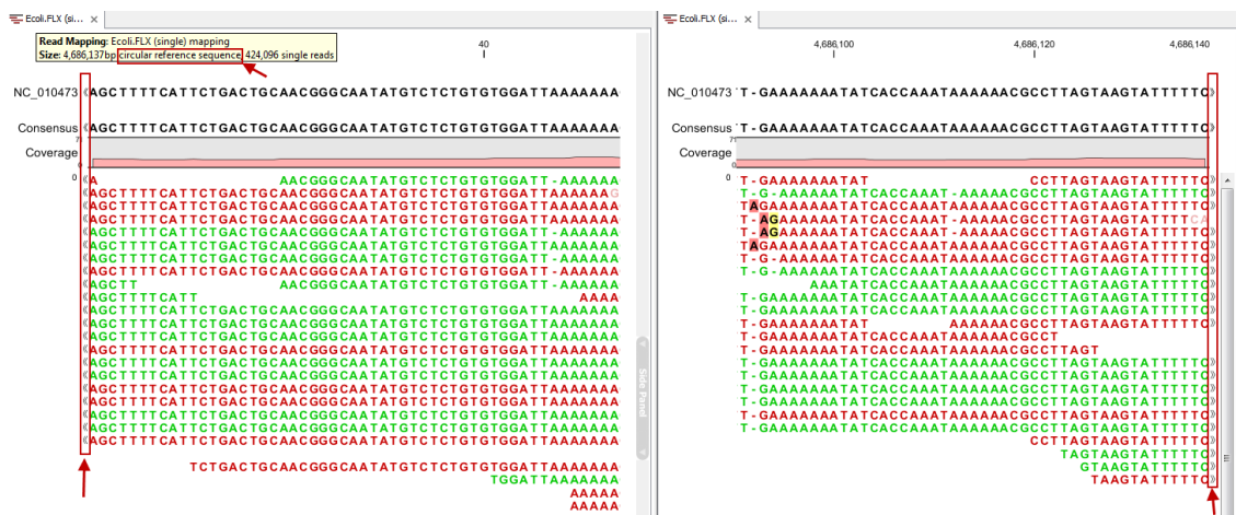
Figure 24.20: Mapping reads to a circular chromosome. Reads that are marked with double arrows at the ends are reads that map across the starting point of the sequence. The arrows indicate that the alignment continues at the other end of the reference sequence.
