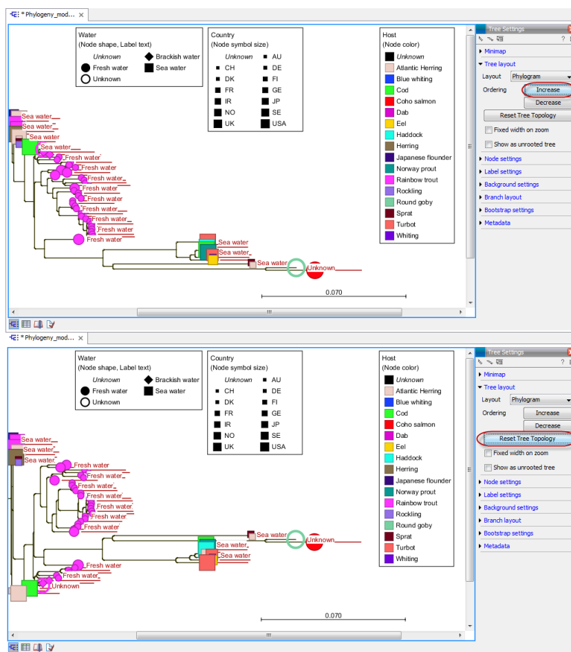
Figure 20.13: The tree layout can be adjusted in the Side Panel. The top part of the figure shows a tree with increasing node order. In the bottom part of the figure the tree has been reverted to the original tree topology.
