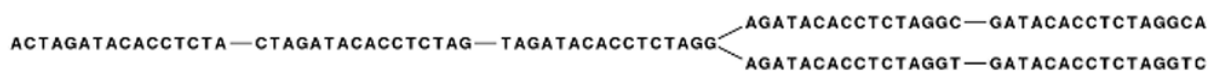
Figure 5.2: Three nodes connected, each sharing 15 bases with its neighboring node and ending with two forward neighbors.
